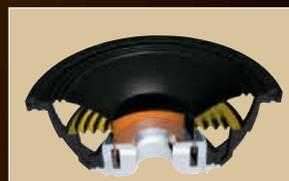
Typical bass units have relatively small voice coils, which, at high power levels, mean reduced power handling ability and loss of efficiency. At a huge 65 mm, the voice coil of the EX Series has considerably greater power handling capability, producing outstanding dynamics, even at high sound levels.
